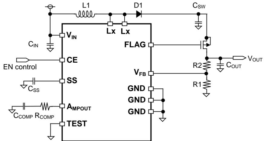
Figure 1. Circuitry with a Complete Shutdown Function
