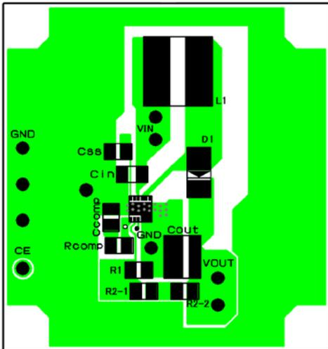
Figure 7. Typical Board Layout – Top Side
