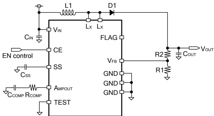
Figure 2. Circuitry without a Complete Shutdown Function
